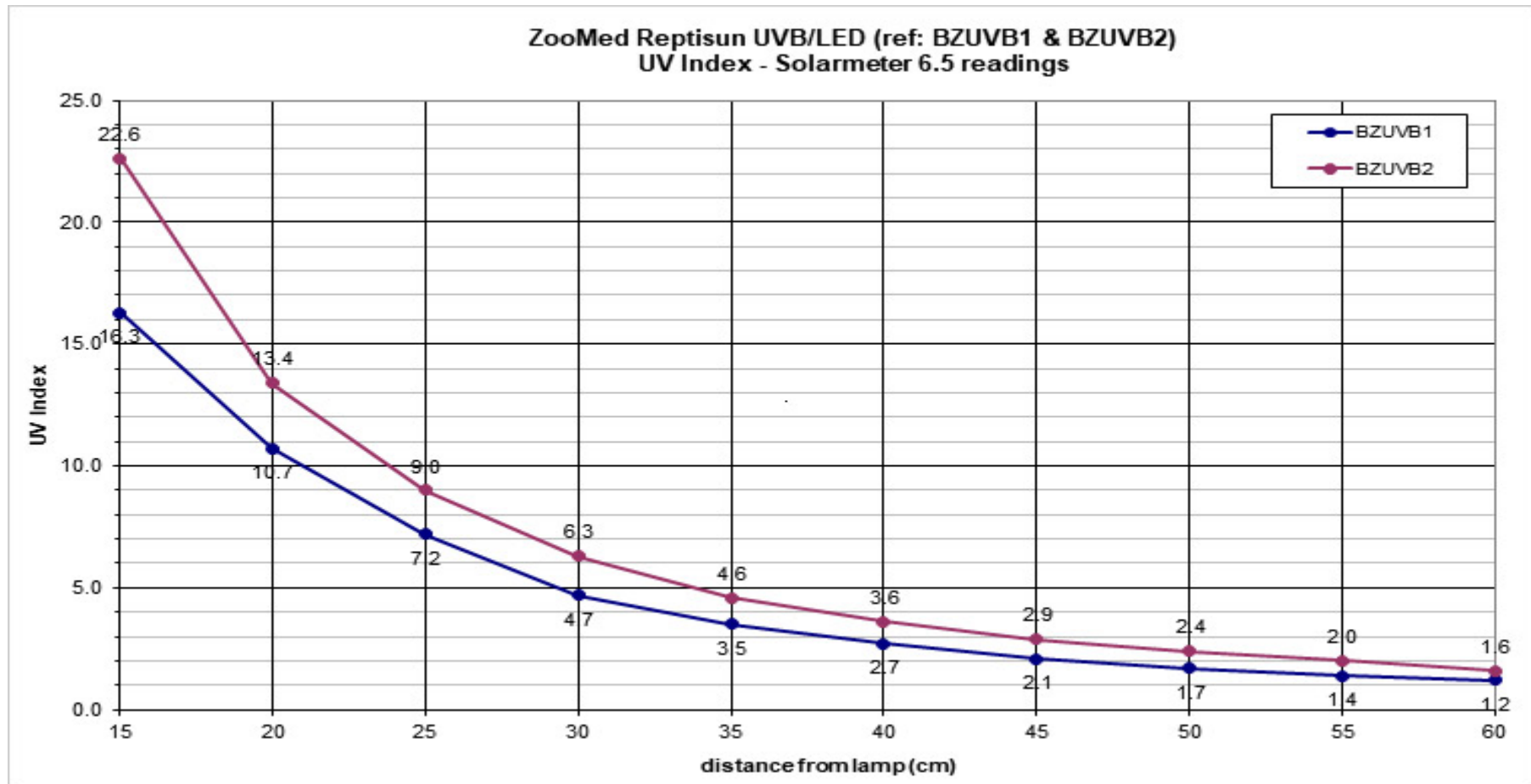
Figure 10 (below) shows the UV Index with increasing distance in graphical form from 15cm to 60cm distance.
