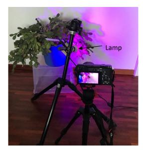
But in a real set-up, there are always objects in the light path. I have put a plant between lamp and a white wall and taken a photo of the illumination at the wall. In a terrarium the total setup will of course be rotated, with the lamp above, illuminating the ground. But as I do not have a white floor and the lamp is too small to use in a terrarium anyway and I only wanted to investigate the effect, I think that this is ok.
