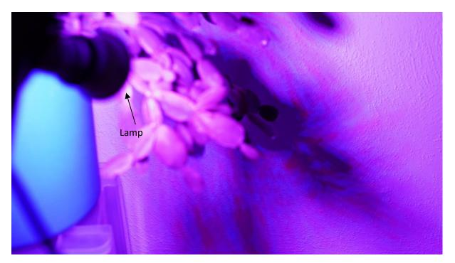
This lamp has 52 red LEDs and 20 blue LEDs that are really closely together and packed in a randomized pattern. There is a big chance that the effects from the individual LEDs are balanced out. It is very unlikely to find a spot at the wall where light from *all* the red LEDs reaches the wall but light from *all* the blue LEDs is blocked by the plant's leaves.
