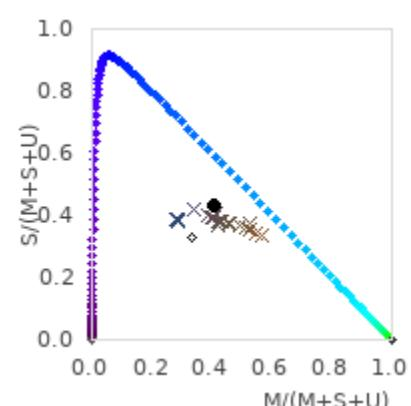
The color of sunlight is also reproduced very well from a reptile's perspective. The color coordinate of the lamp is very close to the color coordinates of different phases of daylight.
